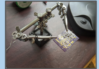
The charge amp board under construction. Each added part is smaller than a grain of rice, ~ 2.00 mm on the longest side
